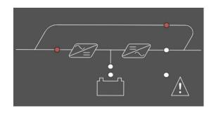
Check the mimic panel to make sure that the device has switched to bypass mode. In this case, the product was transferred to static bypass mode. Loads received from the network is supplied with voltage.
