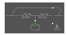
NOTE: the UPS will not switch to normal mode if the inverter voltage is out of limits, or there is an over load or over temperature situation.
