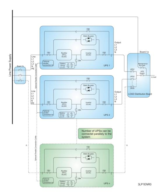
Input and output of more than one UPS are connected to each other; but definitely each battery group is different from another, batteries cannot be used in common. The following points should be considered while placement of UPS in parallel system and their electrical connections are made:
