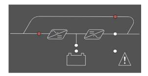
NOTE: UPS will not switch to bypass mode if the inverter voltage is out of limits or there is and overload or overtemperature situation.
