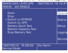
Check the mimic panel to make sure that the device has switched to bypass mode. In this case, the product was transferred to static bypass mode. Loads received from the network is supplied with voltage.
